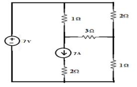
6. a) Explain about Super Nodal analysis and write the steps for applying nodal analysis. [L2][CO1][5M] b) Calculate the current 'I' shown in below figure by using Milliman's theorem. [L4][CO2][5M]
