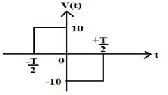
6. a) Find the Trigonometric Fourier series for the waveform shown in figure and sketch the spectrum.[L4][CO4][6M]
