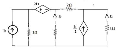
8. a) Derive the expressions for Y-parameters in terms of ABCD parameters.b) Determine the y-parameters of the following network.
