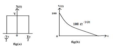
8. Determine the Fourier transforms of the following waveforms shown in figure (a) and figure (b). [L4][CO4][10M]
