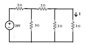
9. a) ) Find the current  $I_{\rm L},$  use millman's theorem as shown in figure below.
