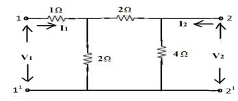
3. a) Explain about h-parameters in terms of y-parameters.b) Find the Short-circuit parameters for the circuit shown in figure.
