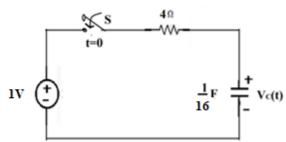
2. a) Derive the Transient Response of series RC-circuit with D.C excitation. [L2][CO3][5M]
